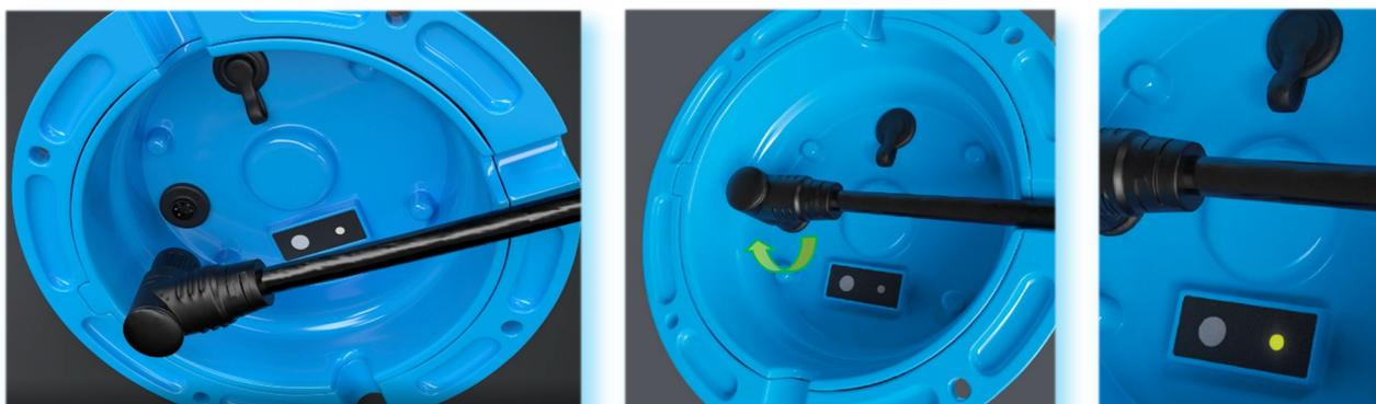
\*\* If the Tank Sender LED flashes **RED** please refer to the “Fault-Finding” section at the rear of this manual.
