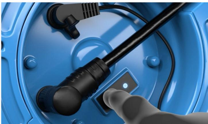
\*\* If the Tank Sender LED flashes **RED** please refer to the “Fault-Finding” section at the rear of this manual.
