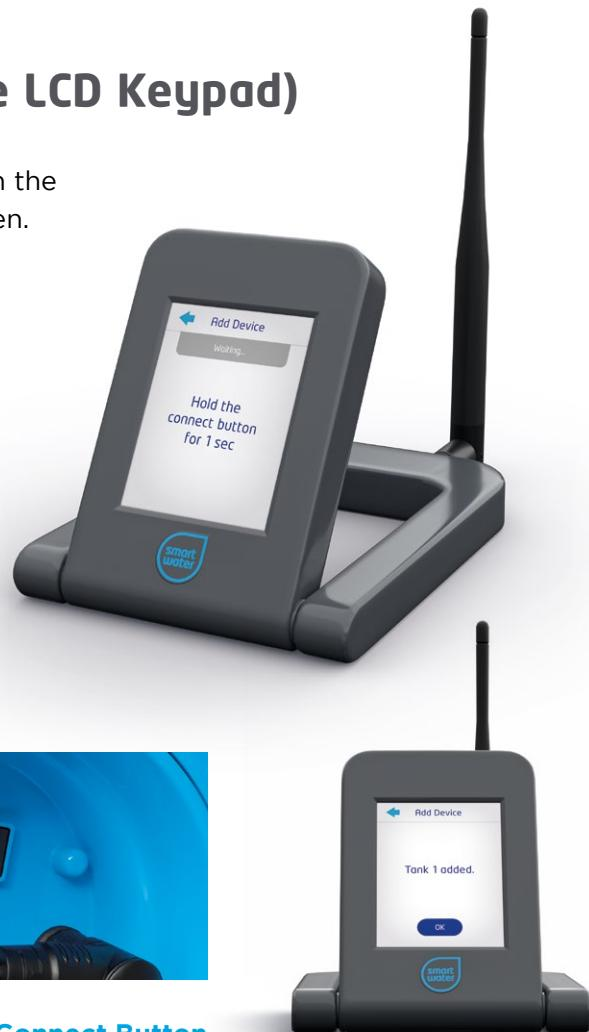
Press and hold the **Connect Button** on the bottom of the **Tank Sender** until the LED illuminates blue for two seconds, followed by two short white flashes.
