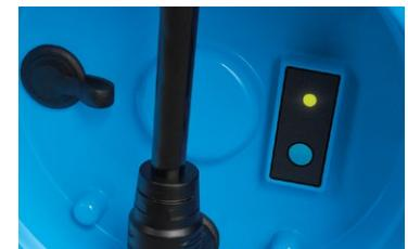
Once the connector is plugged in the LED will flash green until the unit has successfully booted up.
