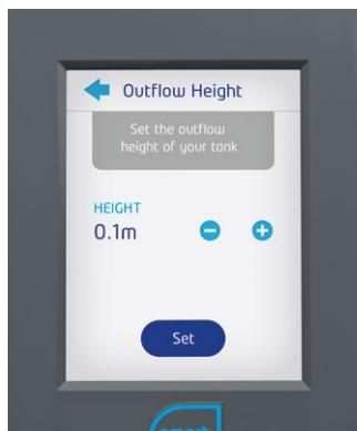
Set your **Outflow Height**. This is the height that water is drained from your tank, normally around 0.1m.
